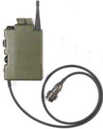
PRR Dual radio with two PTTs and lead to second radio
